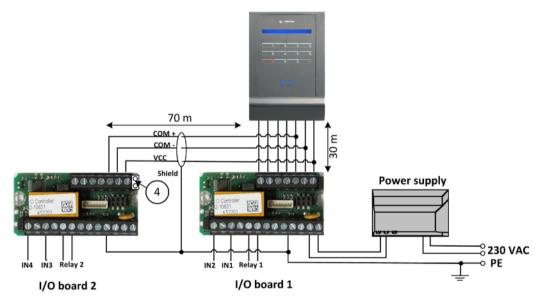
For technical reasons, the total length of the COM cable is limited to 100 m. The length of the COM cable is to be reduced as in the example to ensure that a total length of 100 m is not exceeded. The bridge (4) on I/O controller board 2 must be removed.
