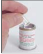
Empty iodine crystals onto metal top of activator canister.
