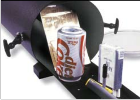
No. CNA2000 FINDER™ packet is used to fume evidence in No. VAC250 CYANOVAC II Fuming Chamber.
